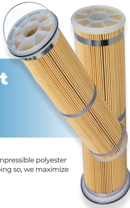
The Polyester Phenolic Treatment (PEPT's) combines the advantages of non-compressible polyester felt with excellent removal of gel-like contaminants into a cartridge format. In doing so, we maximize the available filtration surface area thus extending the life over a bag filter.
