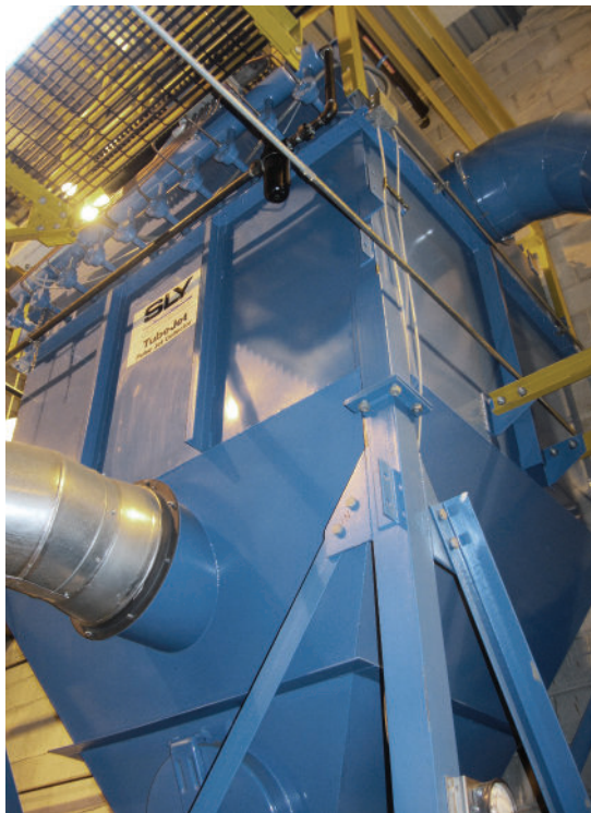
One of six Sly TubeJet collectors utilizing pleated bags at Novamet.
