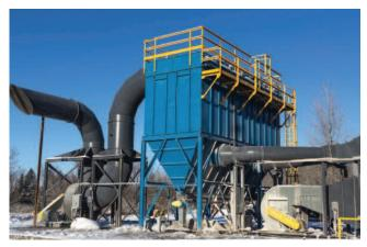
A limestone supplier was looking for a way to meet air pollution emission limits while efficiently and effectively optimizing their production process. The firm needed a way to collect and recycle fines generated from a fluid bed dryer that were released during the drying and cooling process.
