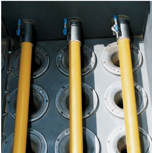
Snap ring filter bags, cages and pulse pipes are removed and installed quickly without tools.
