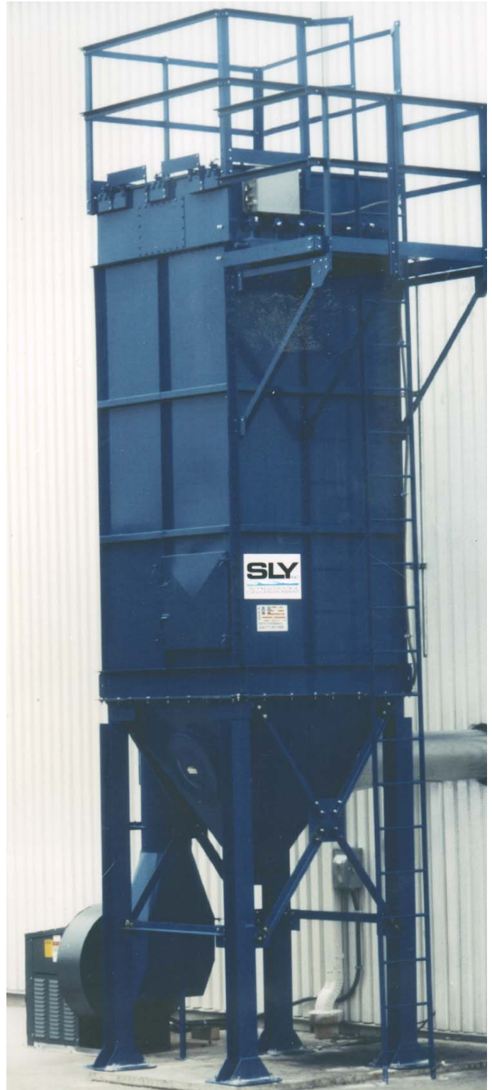
The Sly TubeJet collector offers low cost installation and easy maintenance. It arrives factory-wired, factory-painted (primed inside and out, with an enamel finish on external surfaces), and ready for installation.
