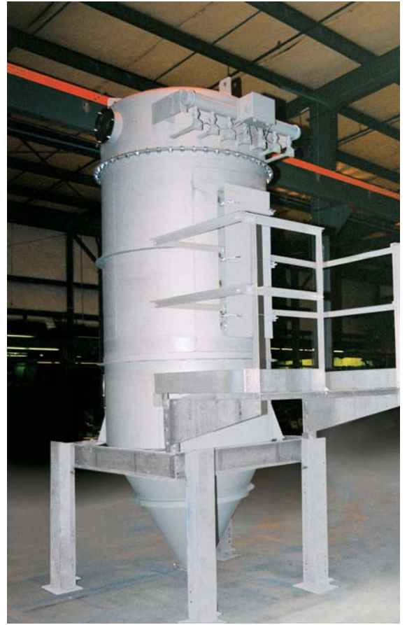
Cylindrical TubeJet collectors are for high pressure/high vacuum applications. All-welded construction permits ranges of \pm 20 " W.G., \pm 100 " W.G., and \pm 17 " Hg. Top or side bag removal styles available.
